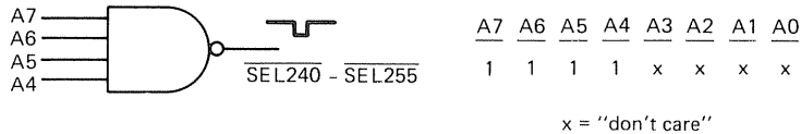
Figure 2-6 Example of a partial decoder. Because address lines A0 through A3 are not used by the decoder, they become "don't cares." The resulting circuit will then decode any address from decimal 240 through decimal 255.
